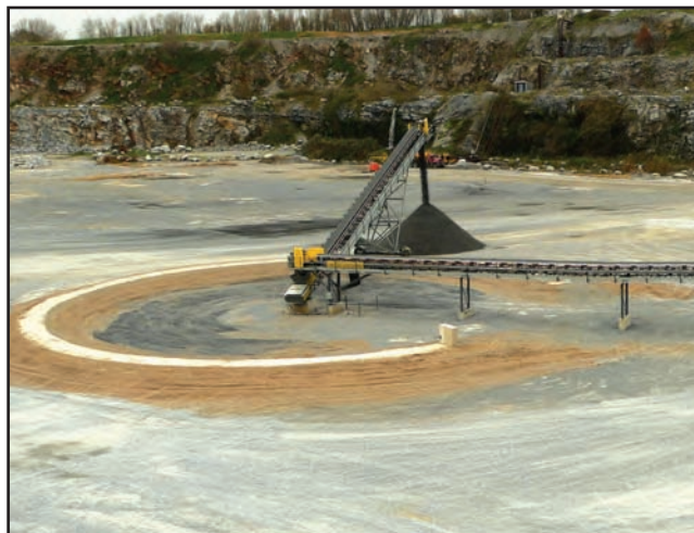
A Steel Systems Equipment-fabricated radial stacker deposits screened aggregate onto a stockpile that can grow to an estimated 50,000 tons in size because of the stackers 270-degrees of travel.
